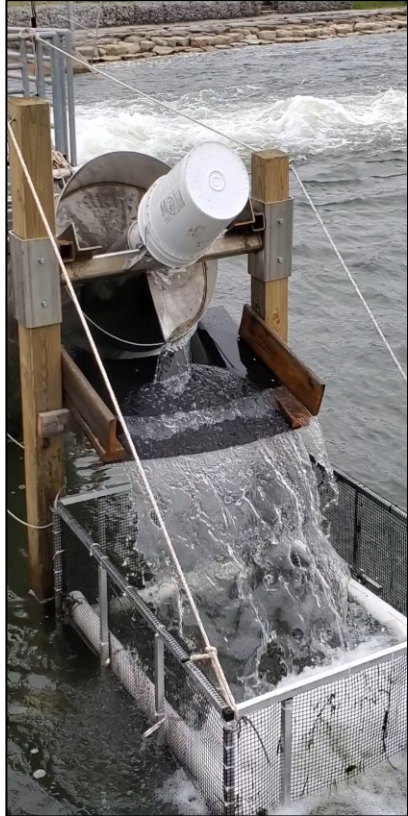
2021: Test of a screw-style fish lift for introducing migratory fish into a selective fish passage device.
