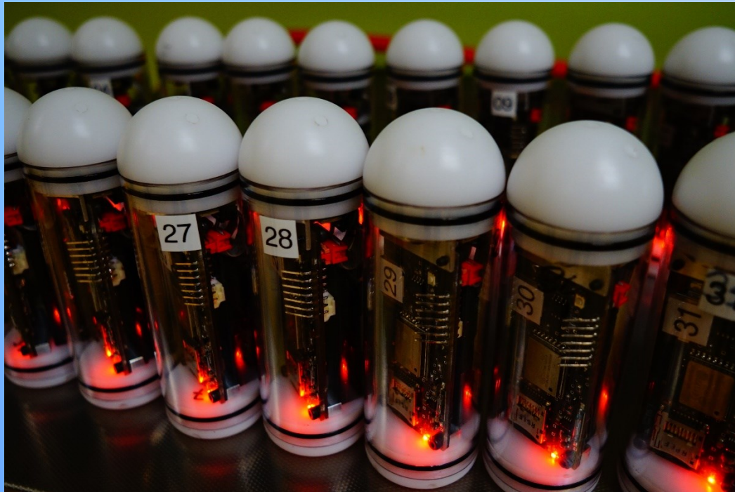
Barotrauma Detection Sensor (BDS)
