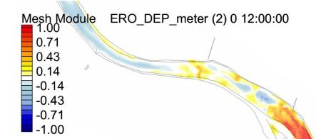
Application of 'morphodynamic' modelling of channel bed evolution as a result of the removal of large weir structure and rock ramp replacement.
